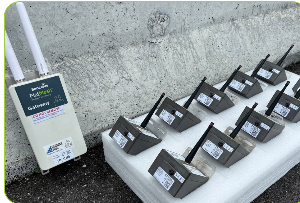
Wireless Triaxial Tilt Sensor nodes and 4G Gateway
